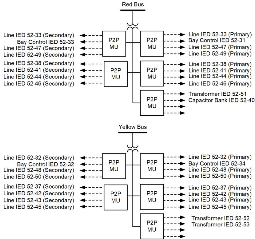
Fig. 9. P2P DSS design for sharing bus voltage.
