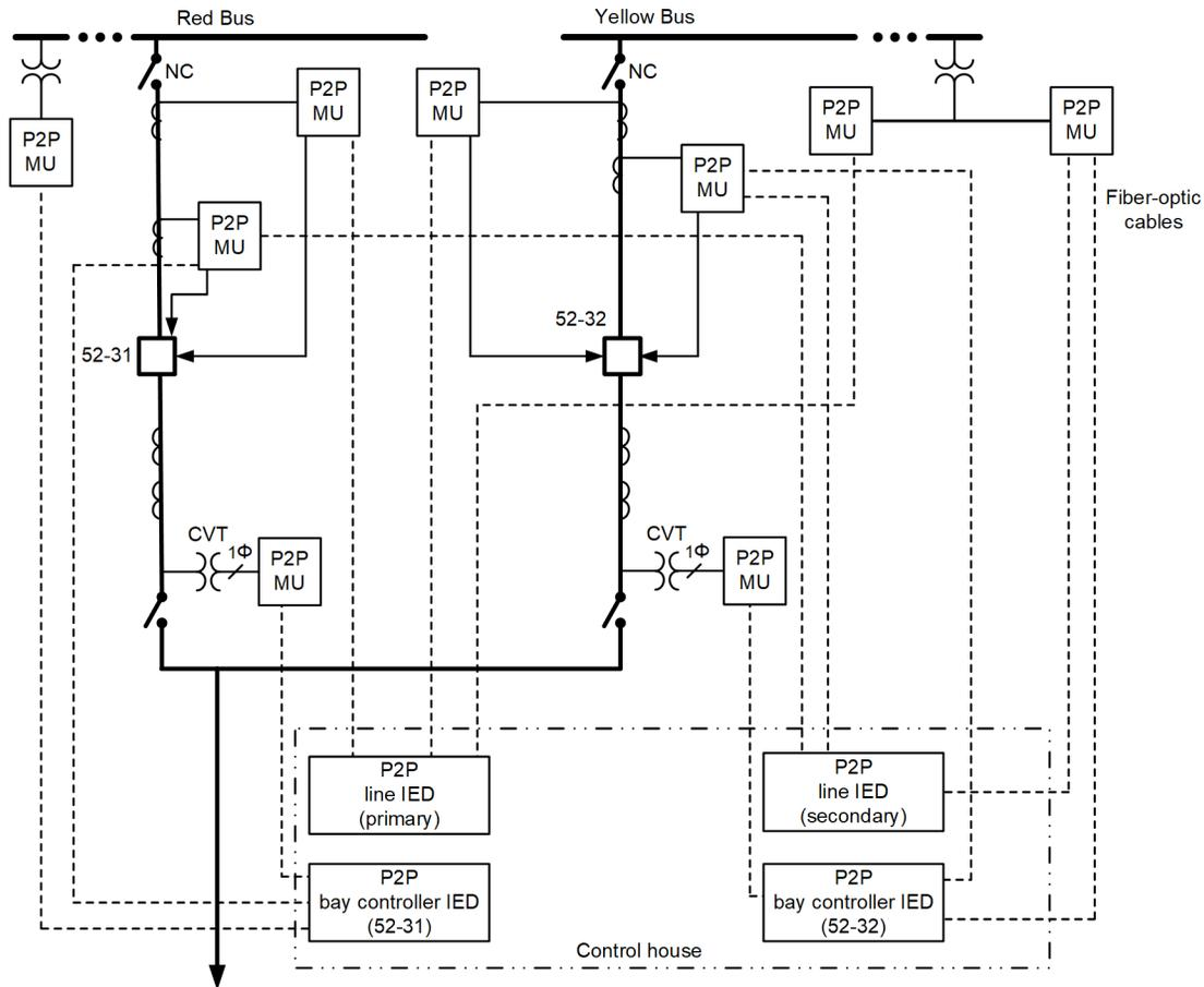
Fig. 4. P2P DSS design for Line 1 protection.
