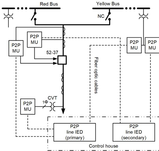
Fig. 6. P2P DSS design for Line 3 protection.
