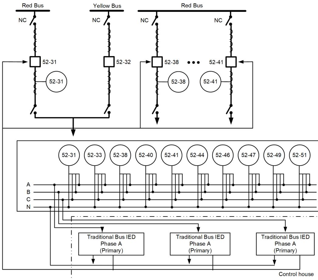
Fig. 7. Traditional secondary connections and IEDs for the Red Bus primary bus differential protection.
