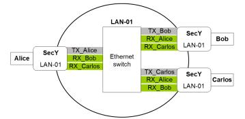
Fig. 2. Illustration of the interaction of MACsec SecYs on a LAN.
