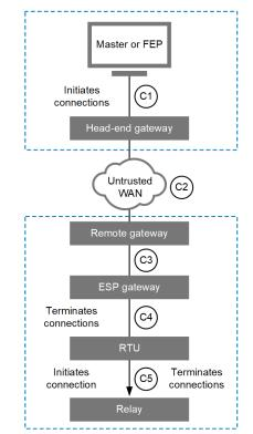
Fig. 18. Substation architecture.
