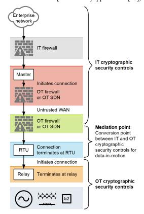
Fig. 15. Example energy system data flow with cryptographic protocol overlay.
