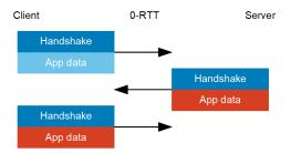
Fig. 14. Packet exchange during 0-RTT TLS initialization.
