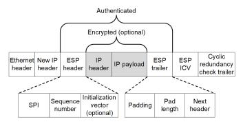
Fig. 9. IP packet encapsulated with ESP tunnel mode.
