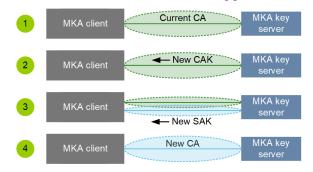
Fig. 8. MKA CAK rotation process.
