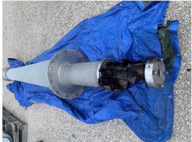
Fig. 24. Removed damaged reactor bushing at Romney.
