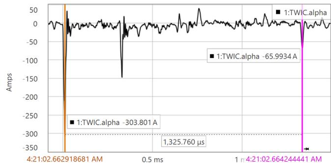
Fig. 33. Sam C-phase alpha-mode current TW arrival times:  $t_1 = 2.662918681$  s and  $t_4 = 2.664244441$  s.
