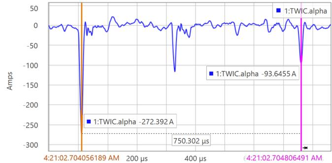
Fig. 32. West Shackelford C-phase alpha-mode current TW arrival times:  $t_1 = 2.704056189$  s and  $t_4 = 2.704806491$  s.
