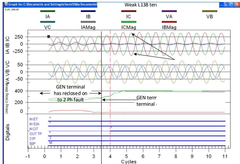
**Figure 26 Record from WEAK terminal after automatic reclose at GEN terminal of L138.**
