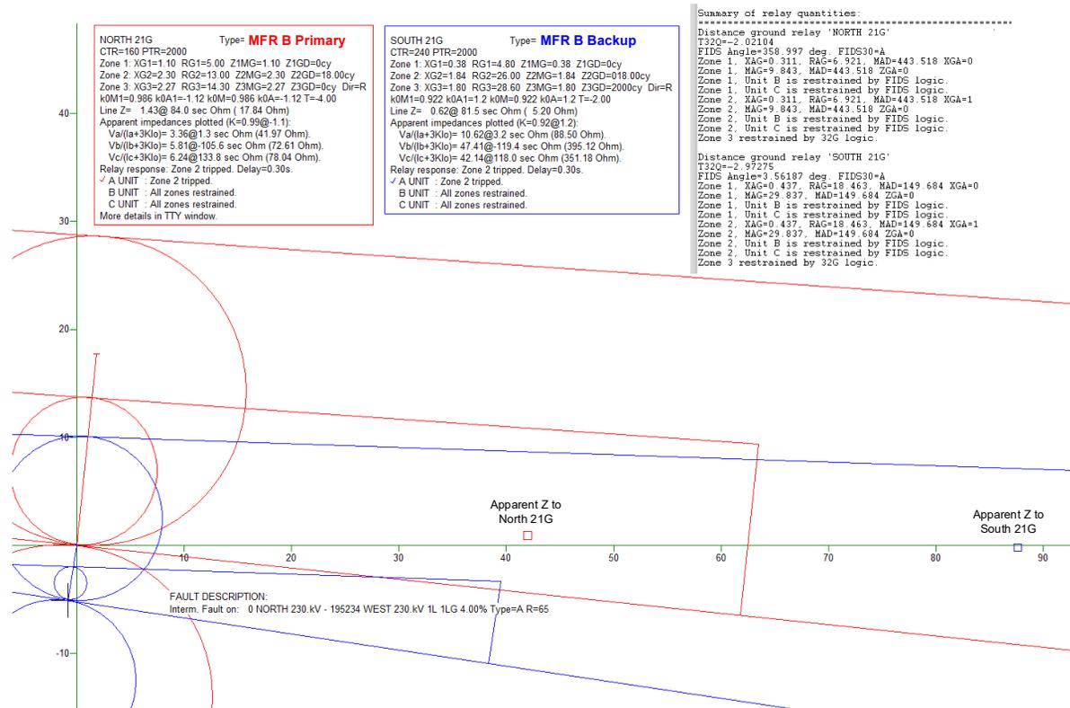
Figure 17 Responses of primary and backup relays to the simulated fault.
