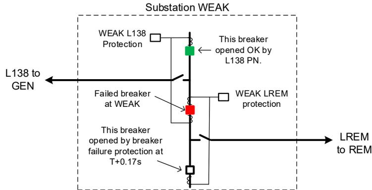
**Figure 23 Single-line diagram of part of Substation WEAK.**
