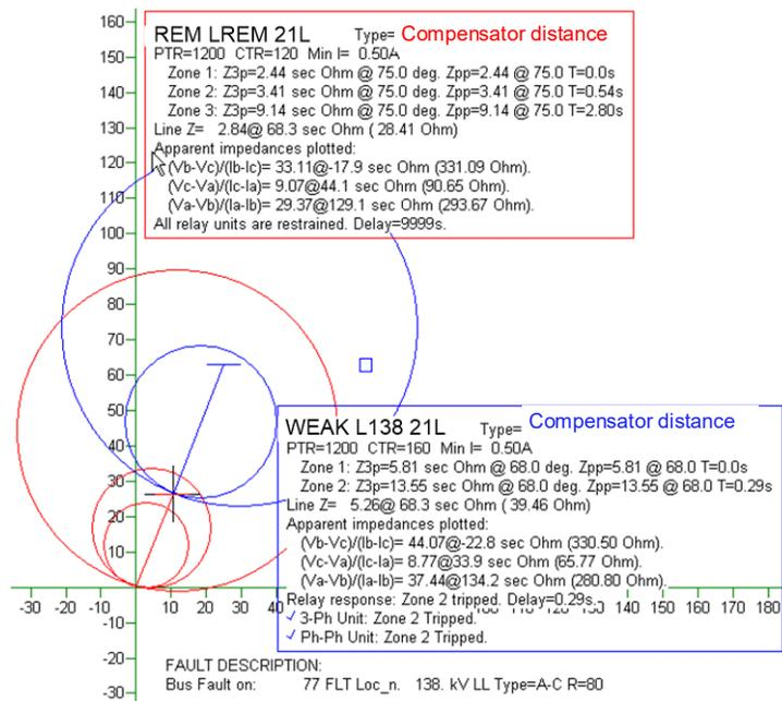
**Figure 27 Responses of WEAK and BACKUP relays after GEN terminal opens a second time.**
