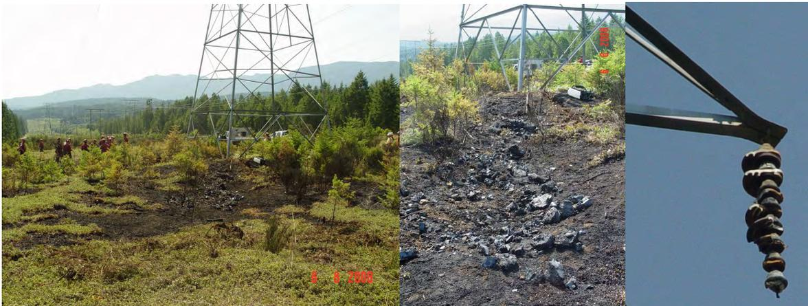
**Figure 3** Aftermath of a 200-ohm 138 kV line 1LG fault.
