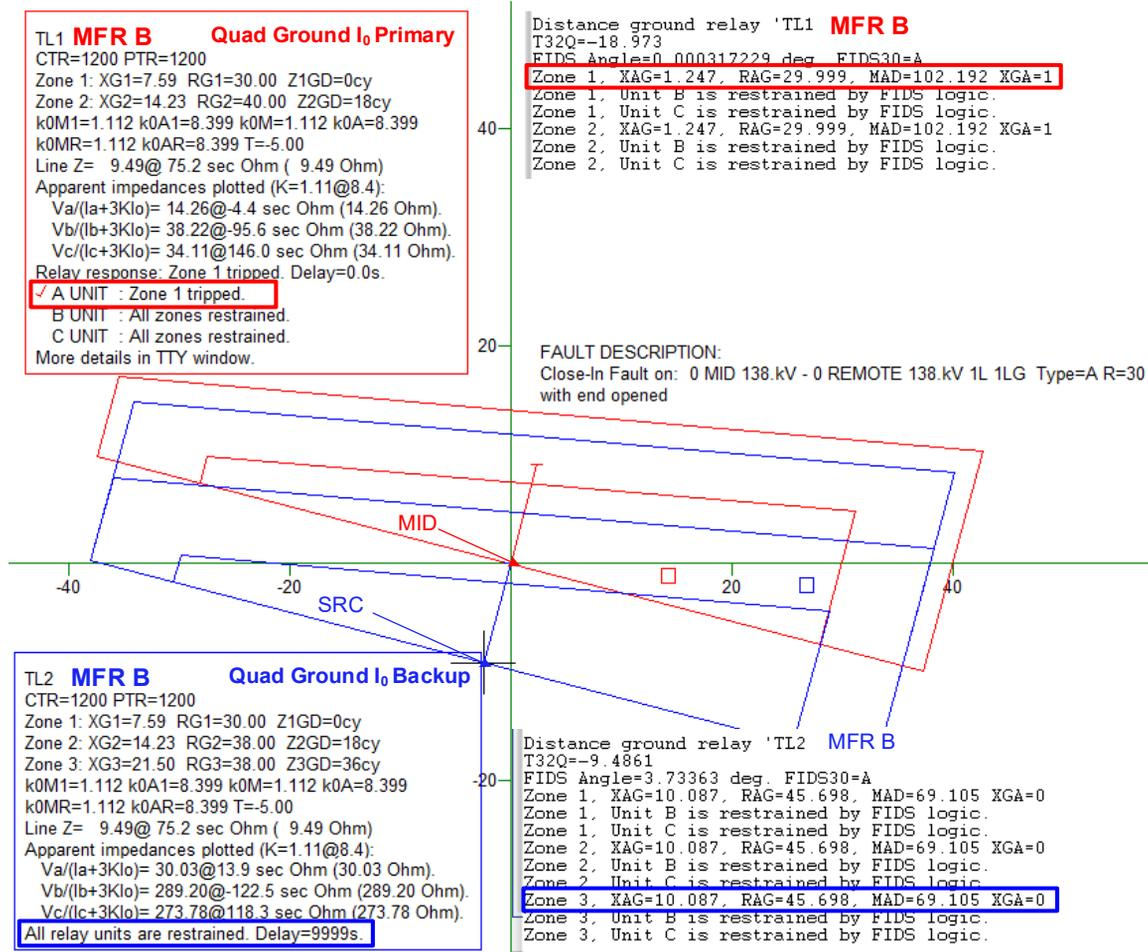
Figure 14 Coordination of ground quadrilateral element considering infeed.
