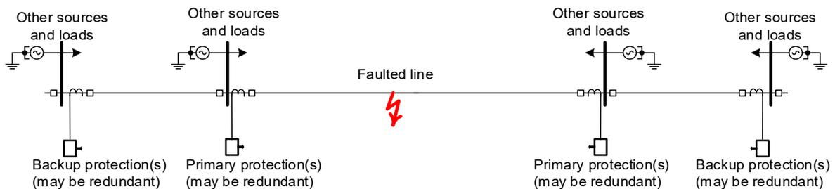
**Figure 1 Example primary and backup protections.**
