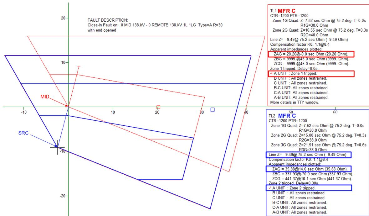
**Figure 15 Coordination of self-polarized quadrilateral element considering infeed.**
