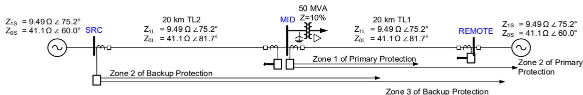
Figure 13 Example system with zero-sequence infeed at MID.
