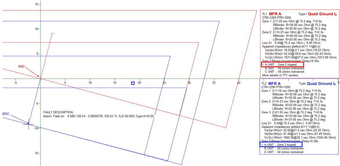
**Figure 9 Zone 2 of the primary and backup relays operates at the same time due to use of different polarizing currents.**
