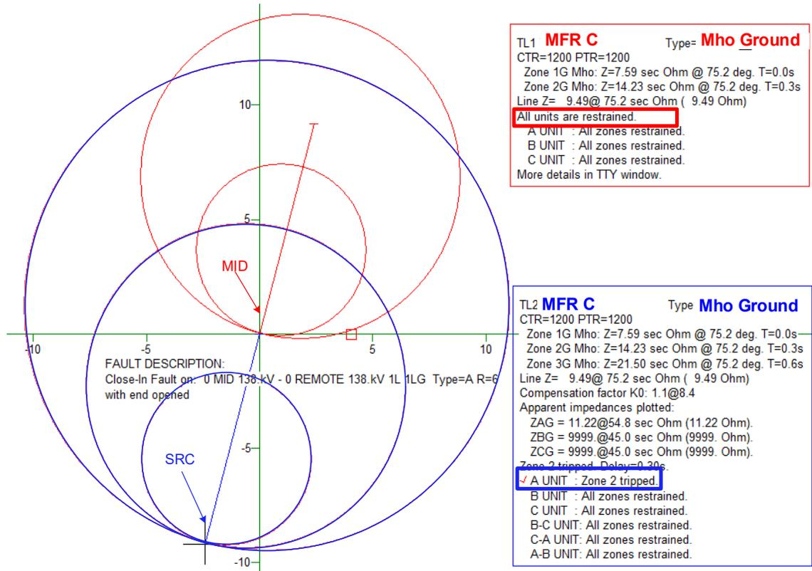
**Figure 10 Primary relay does not trip, whereas backup relay trips for a  $6 \Omega$  1LG fault.**
