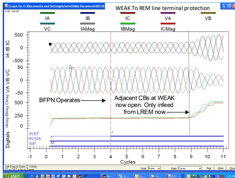
**Figure 24 Infeed to WEAK Terminal from Line LREM at  $T + 0.17$  seconds.**
