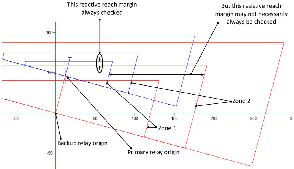
**Figure 2 Coordination margins between a primary and backup relay pair.**
