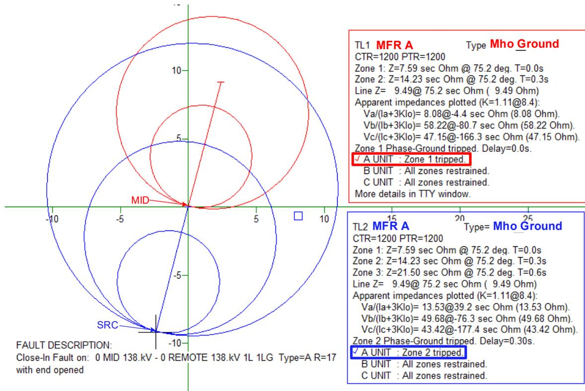
Figure 11 Backup relay coordinates well with primary relay.
