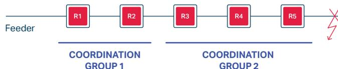
Coordination groups keep time-overcurrent coordination simple and can be applied in any feeder topology.
