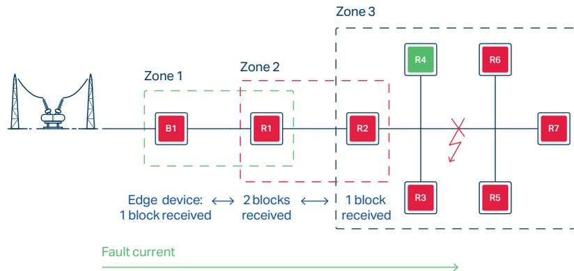
High-speed communications improve fault-clearing times. The HDC scheme remains flexible and can easily accommodate additional reclosers and changes in feeder topology.
