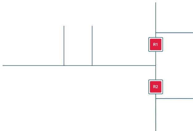
Feeder networks are evolving. Advanced power grids increase the number of reclosers to reduce the number of customers in each line segment.
