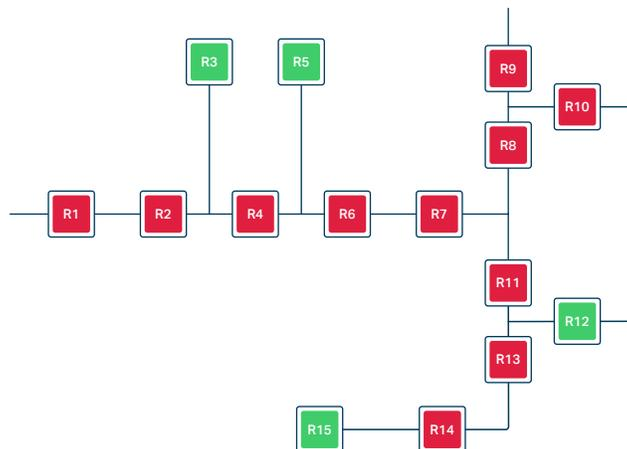
SEL HDC simplifies the protection scheme, allowing practically any number of reclosers to operate selectively within coordination margins.
