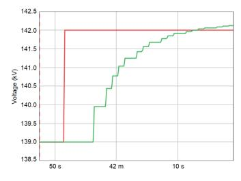
Fig. 3. 1 s data update with a 3 kV voltage response
