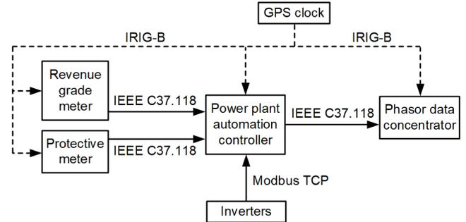
Fig. 1. Example of phasor communication architecture for power plant control
