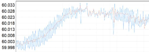
Fig. 2. Frequency measurements in IEEE C37.118.1-2011 (orange) vs. IEEE C37.118.2005 (blue)
