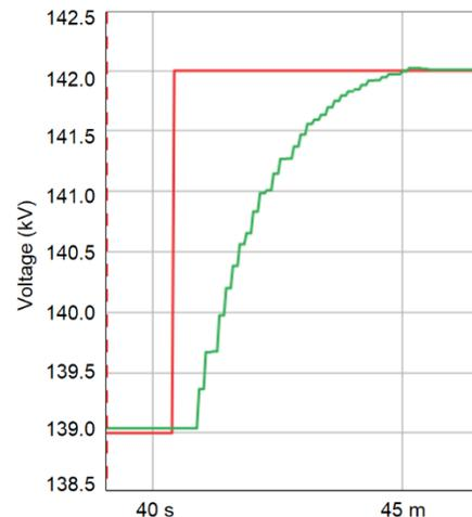
Fig. 4. 100 ms data update with 3 kV voltage response
