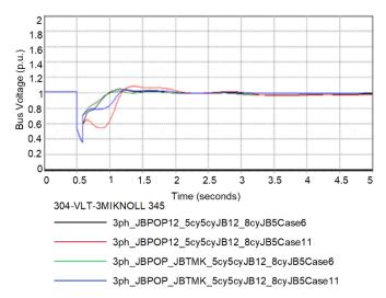
Fig. 7. Threemile Knoll 345 kV voltage for N–2 outage or 345 kV lines west of Jim Bridger.
