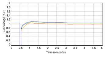
Fig. 8. Voltage performance of tripping wind versus Jim Bridger units to determine effectiveness factor.
