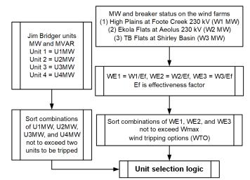
Fig. 4. Inputs to unit selection logic.
