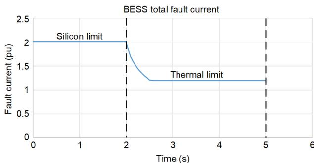
Fig. 5. Specified BESS current capability curve
