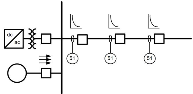
Fig. 7. Grid-connected overcurrent coordination
