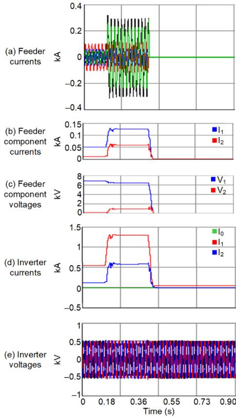
Fig. 11. Distribution feeder Phase-A-to-ground fault (islanded operation)
