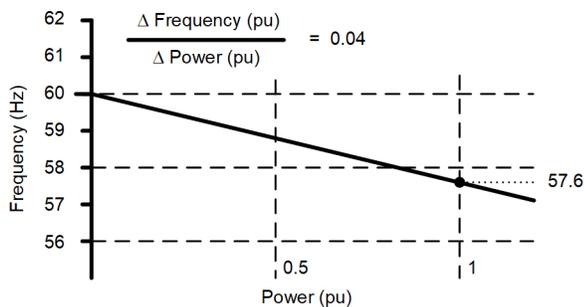
Fig. 3. Four percent frequency droop curve
