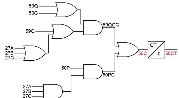
Fig. 8. 50C—voltage-controlled overcurrent
