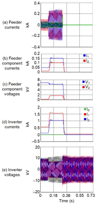
Fig. 12. Distribution feeder Phase-B-to-C fault (islanded operation)
