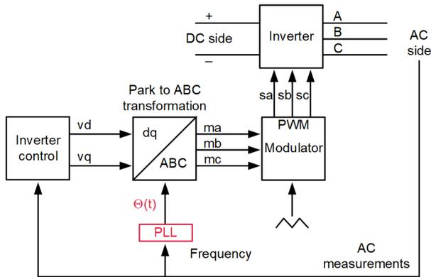
Fig. 2. GFL-PLL-based inverter requires strong voltage source
