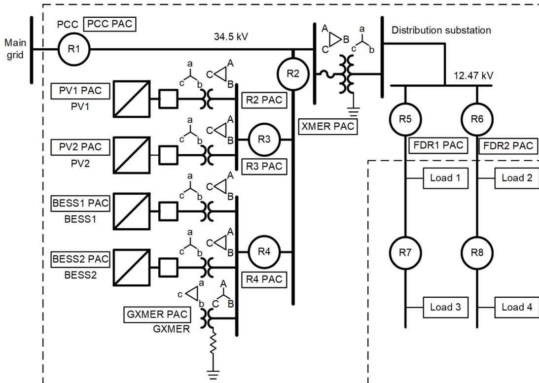
Fig. 6. Solar-plus-storage project configuration
