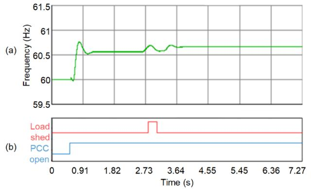
Fig. 13. Loss of the PCC (utility) and load shedding
