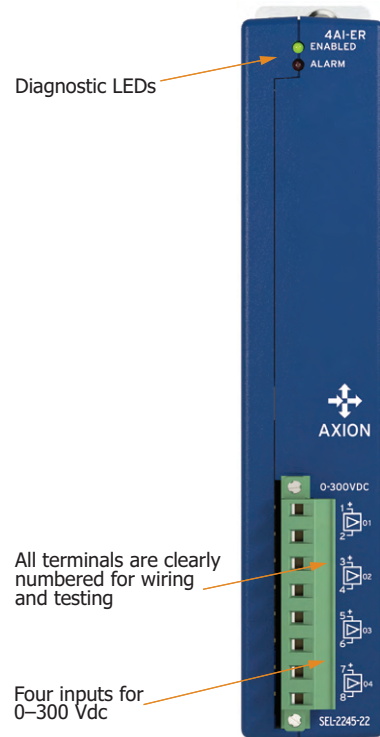
Figure 10 SEL-2245-22 Analog Input Extended Range Module Terminal-Side View
