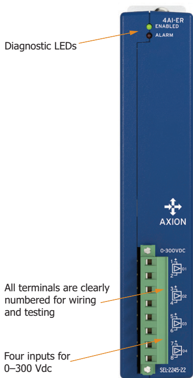
Figure 12 SEL-2245-22 Analog Input Extended Range Module Terminal-Side View
