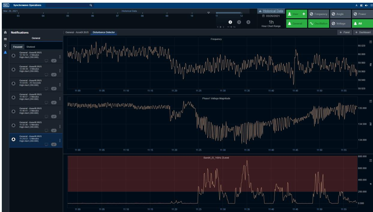
Example Oscillation Event Analysis Dashboard Showing Disturbance Detector Results
