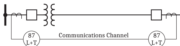
Figure 19 In-Line Transformer With Combined Line and Transformer Current Differential
