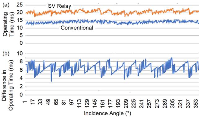
Fig. 9. (a) Comparison of operating times for various points of incidence. (b) Time difference between the two solutions in relation to the point of incidence: three-pole tripping.
