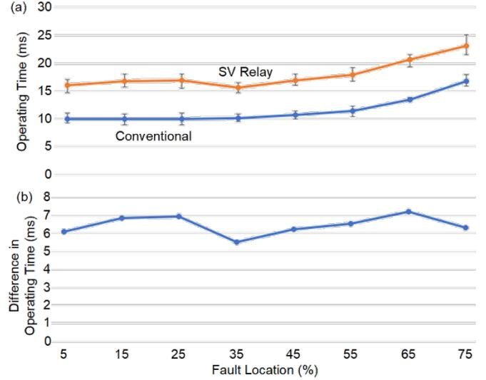
Fig. 3. (a) Operating times of the two solutions evaluated for several fault locations. (b) Average difference in operating times for different fault locations between solutions.
