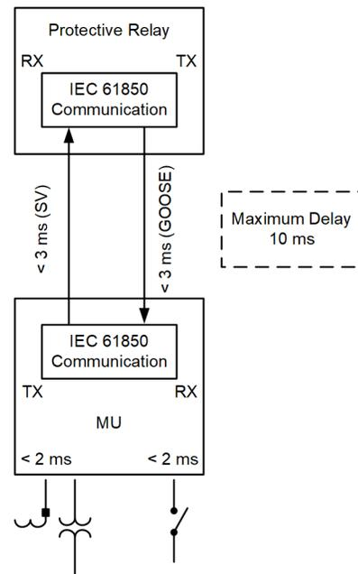
Fig. 2. Requirements for speed of communication between IEDs.
