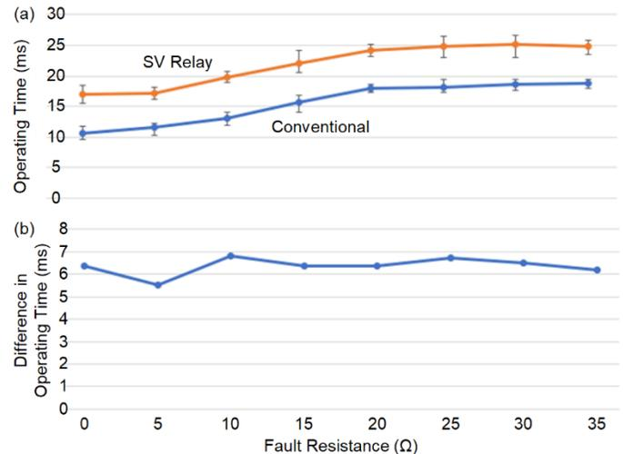
Fig. 12. (a) Operating times as a function of fault resistance. (b) Difference in operating time as a function of fault resistance.
