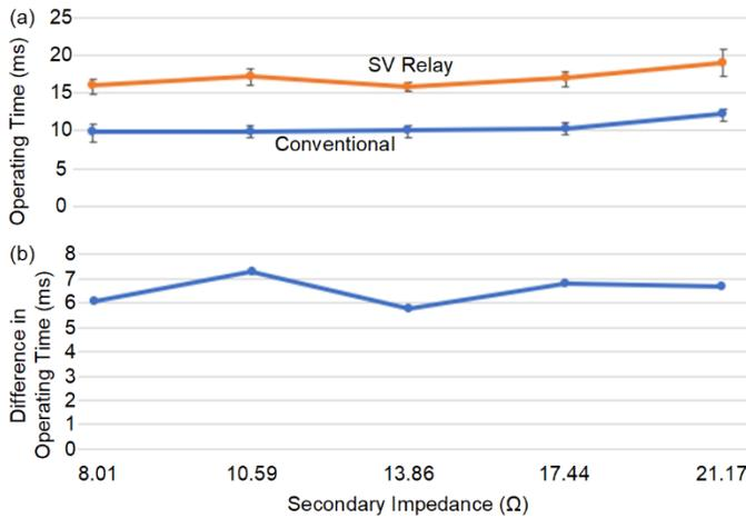
Fig. 13. (a) Operating time in relation to CT secondary impedance. (b) Difference in operating time in relation to CT secondary impedance.
