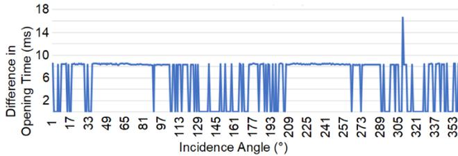
Fig. 5. Differences in breaker opening times: single-pole tripping.
