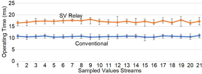
Fig. 17. Operating times compared to the number of streams on the network.
