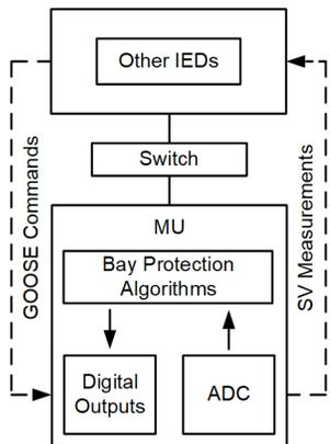
Fig. 18. MU with protection elements.
