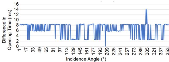
Fig. 10. Differences in breaker opening times: three-pole.
