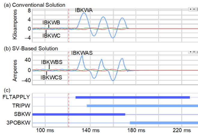
Fig. 14. Fast operation of conventional relay even with CT saturation.
