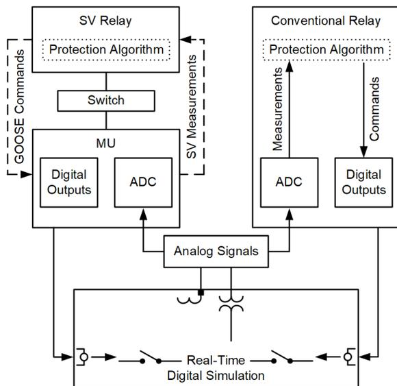
Fig. 1. Test diagram: SV solution on the left, conventional solution on the right.
