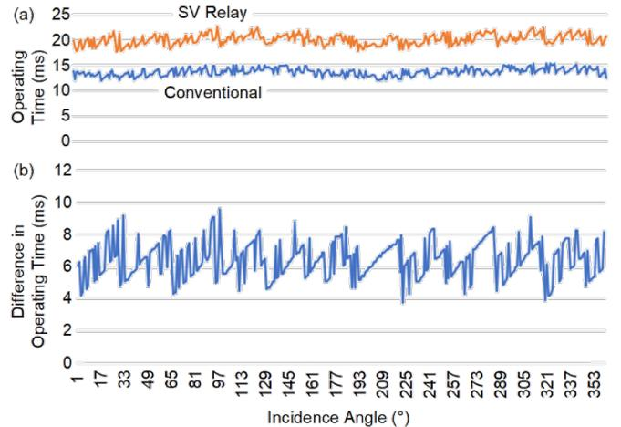
Fig. 4. (a) Comparison of operating times for various points of incidence. (b) Operating time difference between solutions in relation to the point of incidence: single-pole tripping.
