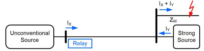
Fig. 2. External fault behind the remote terminal.
