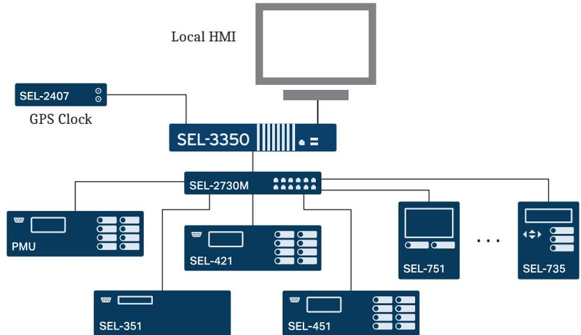
**Figure 5 System Control and Synchrophasor Data Concentration**
