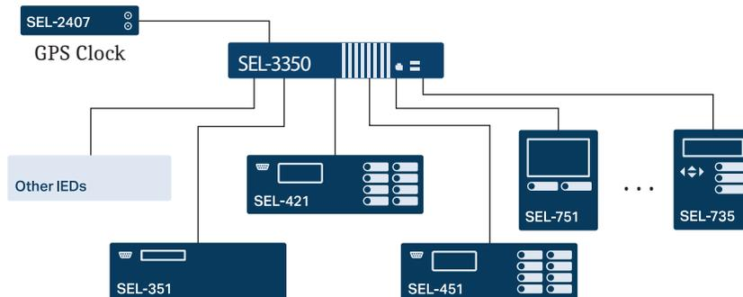
**Figure 4 Distribute Time With Serial Communications Cable**
