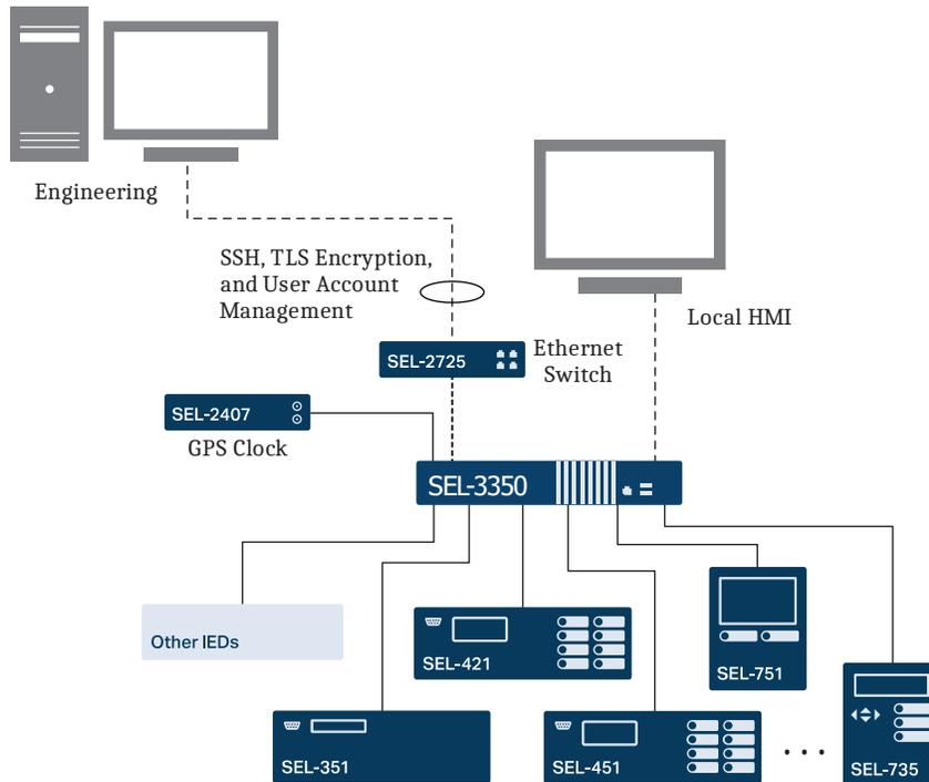
**Figure 2 Engineering Communication Through a Network Access Point**
