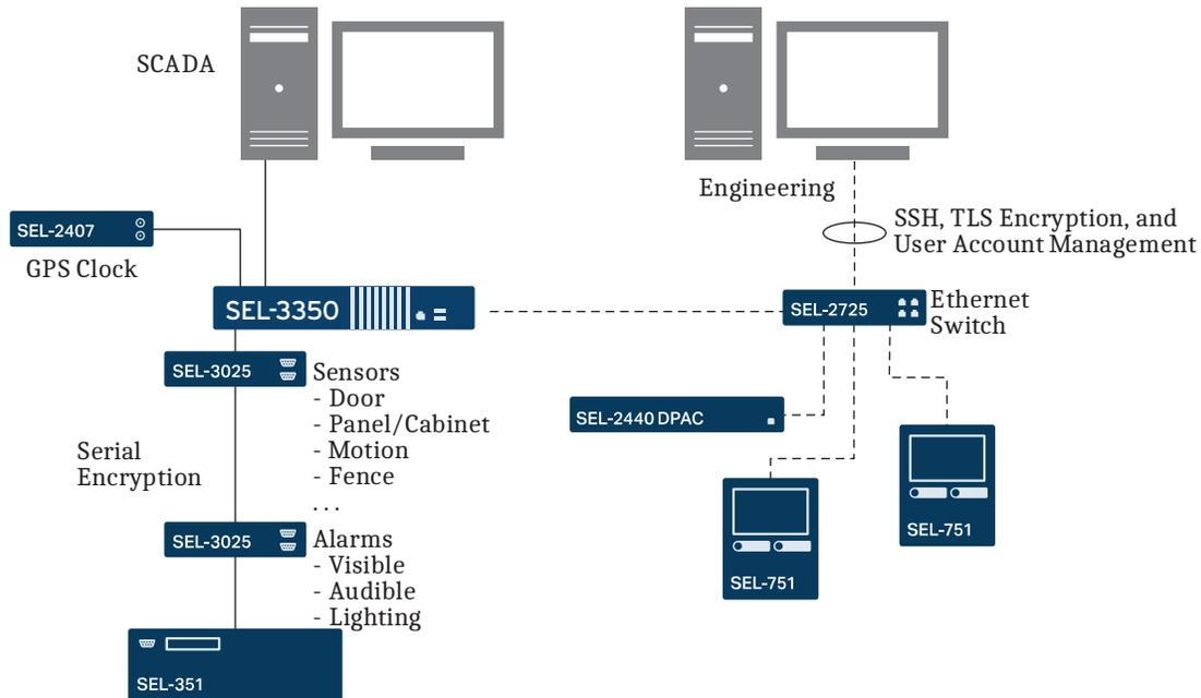
**Figure 7 Security Through a Single Access Point**
