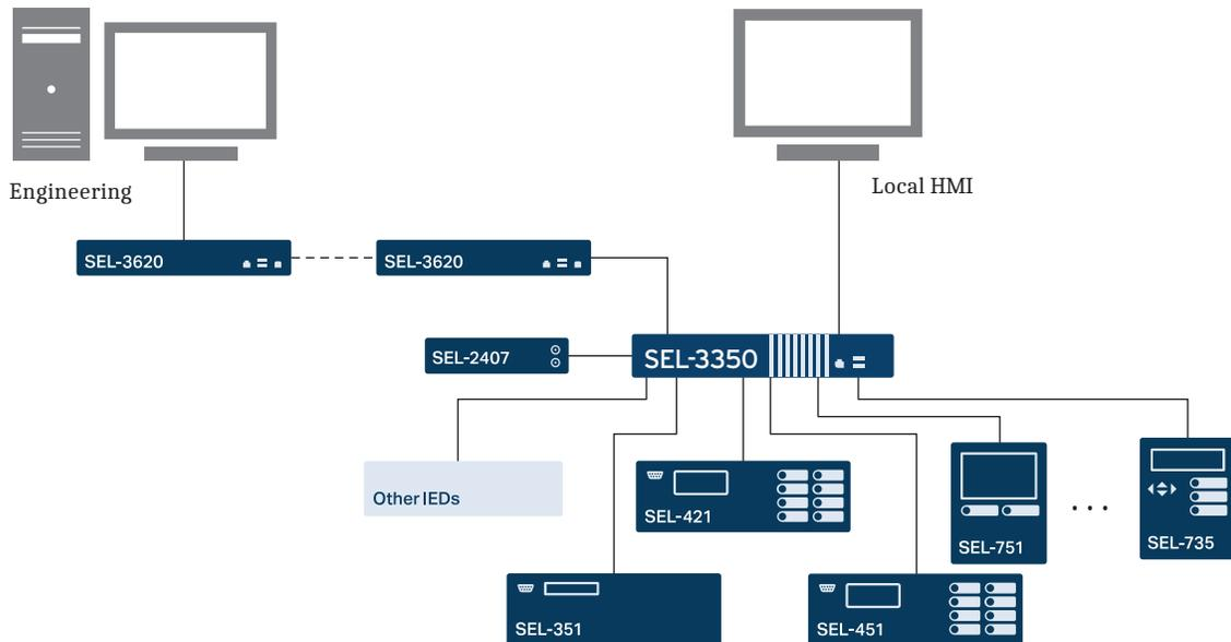
**Figure 1 Engineering Communication Through a Serial Access Point**
