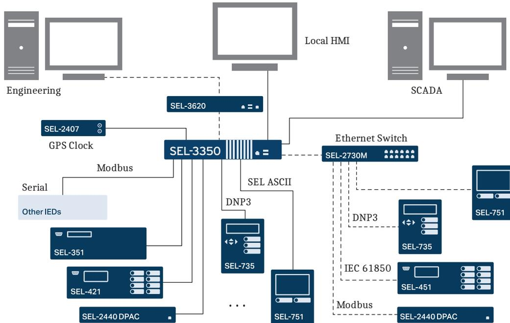
**Figure 6 SCADA Communication Through a Single Access Point**
