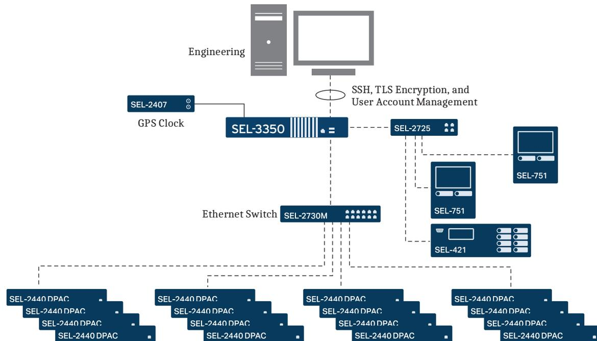
**Figure 8 Automate and Integrate With Communication and Logic**
