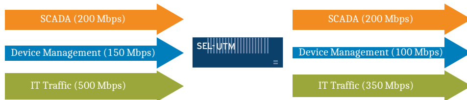
Figure 4 Using Traffic Shaping to Prioritize OT Traffic
