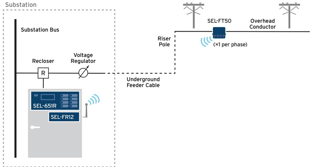
Figure 6—Distribution substation application overview with the SEL-FT50 and SEL-FR12 system.
