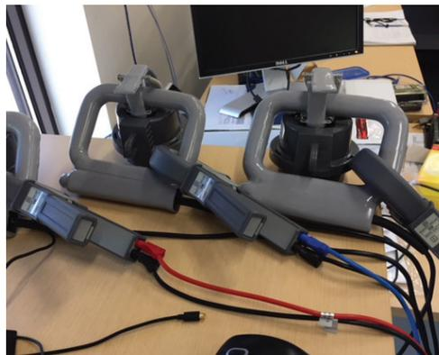
Figure 4—MCL120 current loops connected to SEL-FT50 transmitters in the test lab.
