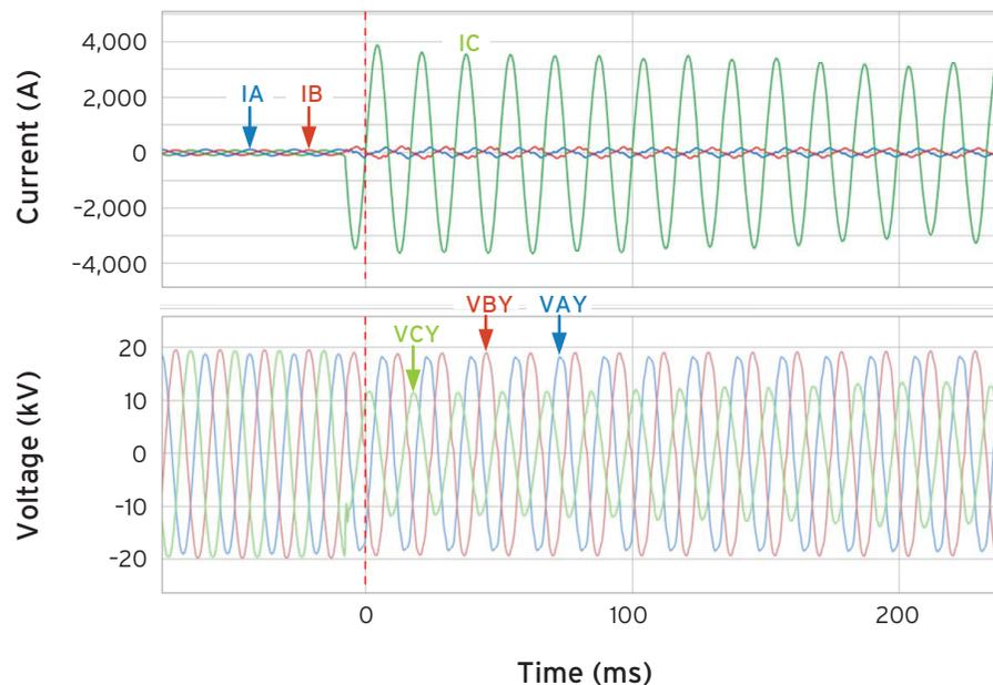
Figure 10—Oscillography from the SEL-651R showing the inception of a fault on Phase C.
