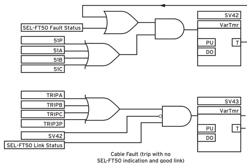
Figure 3—SEL-651R relay logic programming defines how it will use status indication from each transmitter.
