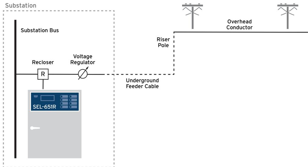
Figure 2—Simplified one-line diagram of the Northside substation at Clayton Public Power.
