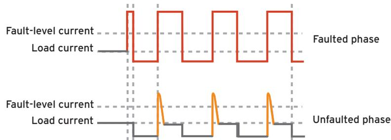
Figure 1—Simplified example of typical automatic reclose sequence.
