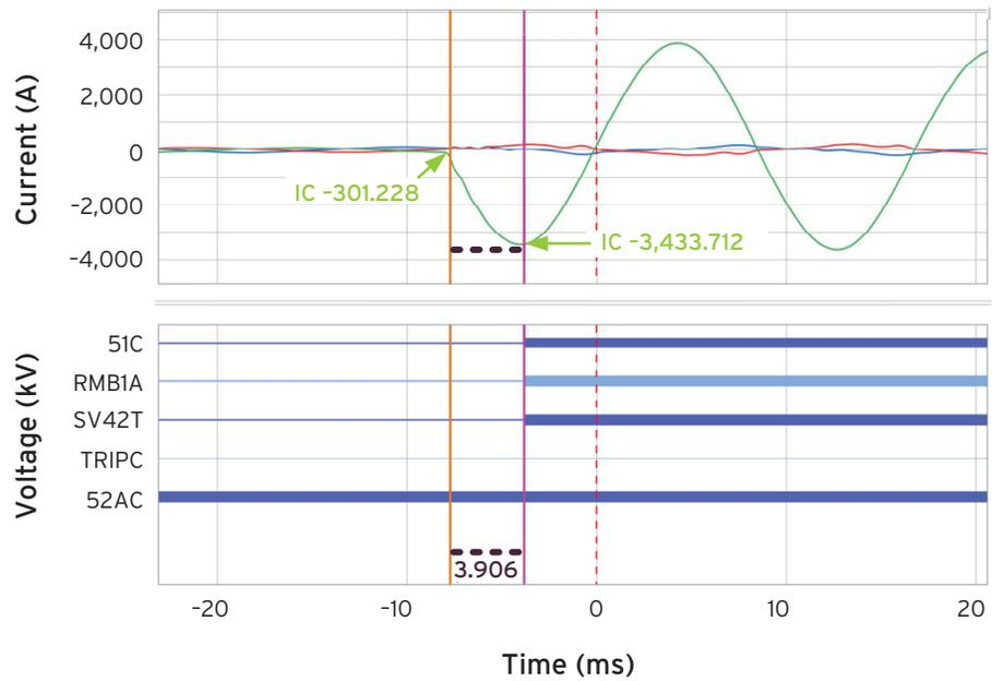
Figure 11—The assertion of the SEL-FT50 fault status Mirrored Bit from the SEL-FR12 approximately 4 ms after the fault inception.
