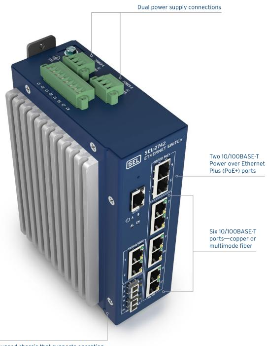
Rugged chassis that supports operation from -40° to +85°C (-40° to +185°F) and meets the IEEE 1613 standard
