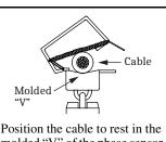
molded "V" of the phase sensor housing.
