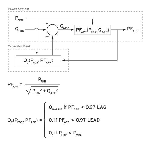
Figure 4—PF control block diagram.
