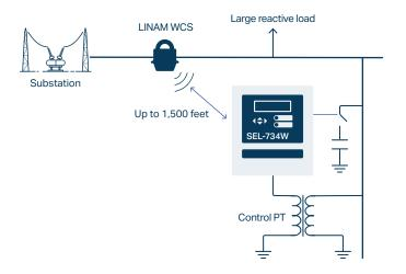
Figure 9—The LINAM WCS provides current measurement of feeder to SEL-734W installed on lateral tap.
