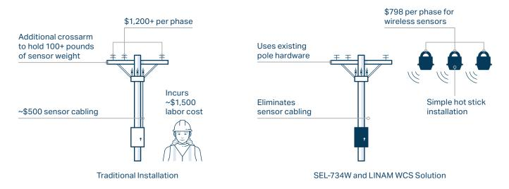
Figure 8—Cost comparison between a traditional installation and the SEL-734W and LINAM WCS solution.
