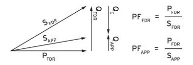
Figure 1—Capacitor bank contribution to power triangle.
