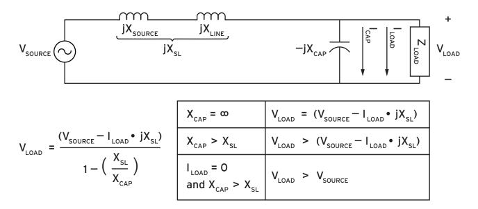
Figure 2—Capacitor bank contribution to voltage.
