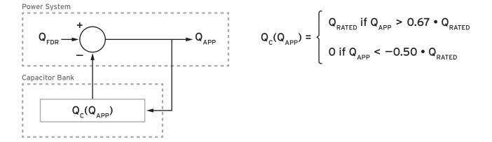
Figure 3—VAR control block diagram.
