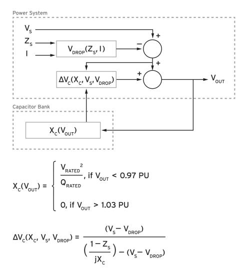
Figure 5—Voltage control block diagram.
