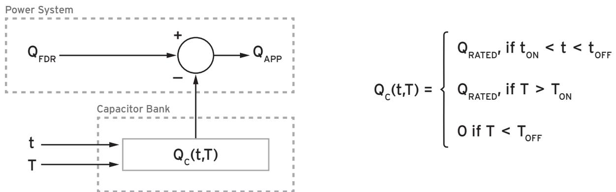
Figure 6—Time-and-temperature control block diagram.
