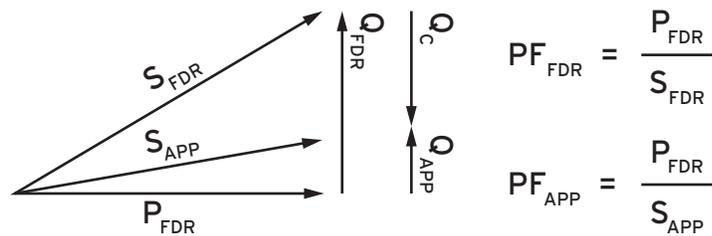
Figure 1—Capacitor bank contribution to power triangle.
