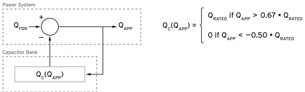
Figure 3—VAR control block diagram.
