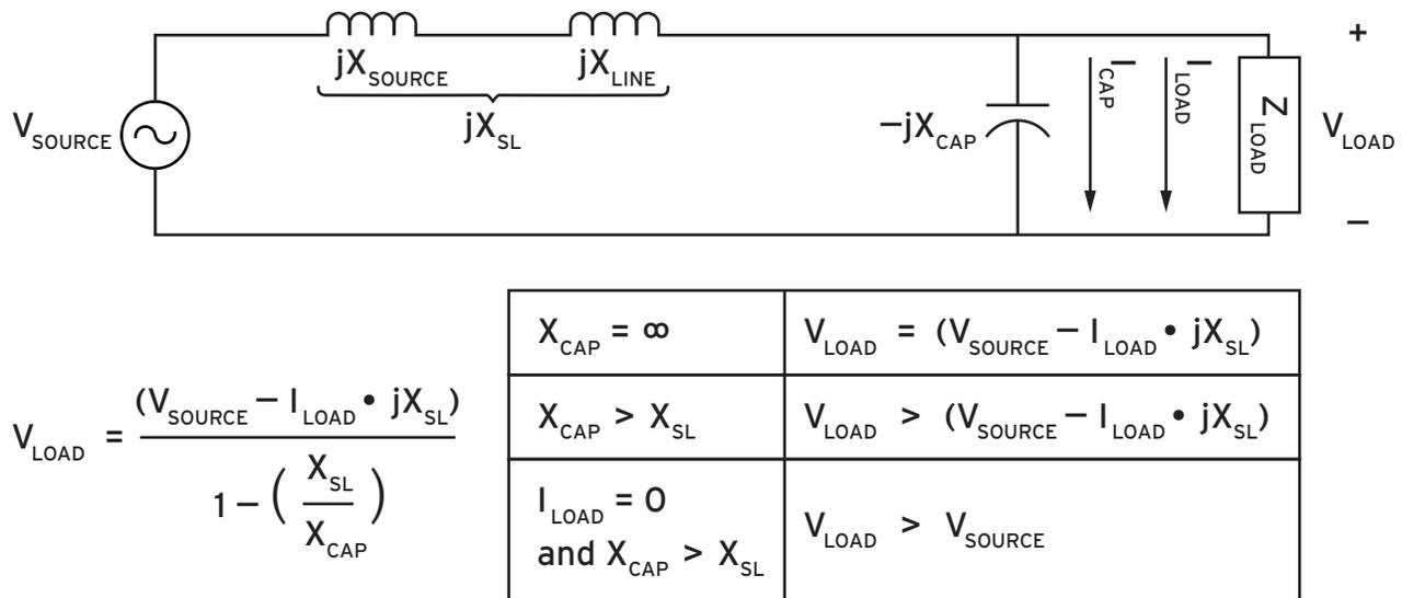
Figure 2—Capacitor bank contribution to voltage.
