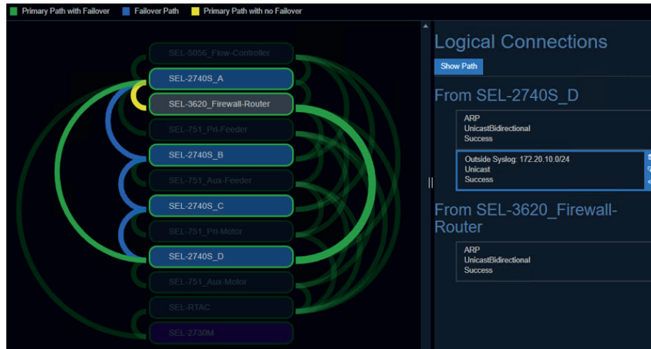
Figure 4—Logical connection allowing “SEL-2740S_D” to send Syslog messages to an outside network through the SEL-3620.
