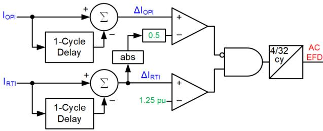
Fig. 4. AC EFD logic.
