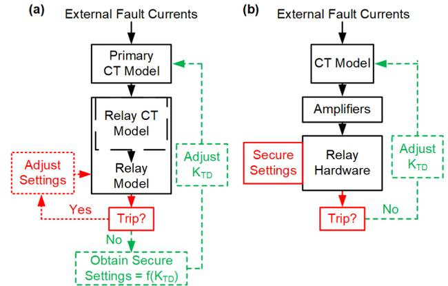
Fig. 7. Determining CT requirements via model (a) and hardware-in-the-loop tests (b).
