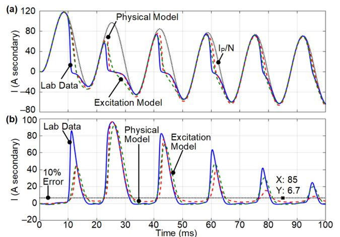
Fig. 2. Comparison of laboratory data and models using secondary currents (a) and excitation current (b).
