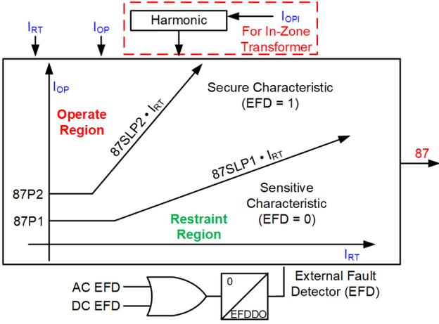
Fig. 3. Characteristic of a differential relay zone.
