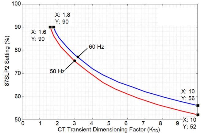
Fig. 8. Application guidance for the differential element without remanence.
