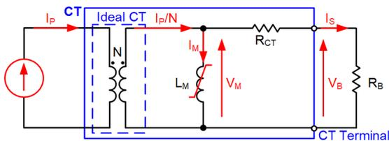
Fig. 1. Equivalent circuit of a CT.
