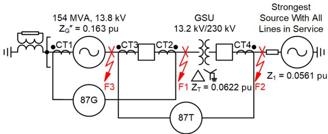
Fig. 9. Example system used to demonstrate CT sizing with all impedances referenced to the generator ratings.
