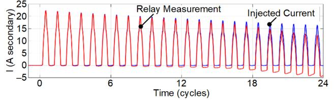
Fig. 6. Relay internal CT response for a unipolar inrush.
