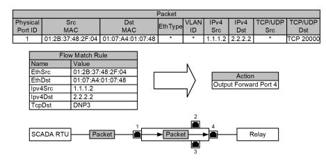
Fig. 8. Packet Forwarding Via Flow Match Rule
