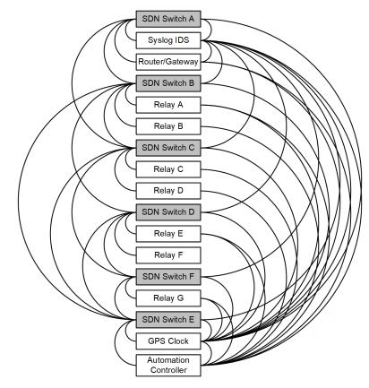
Fig. 10. SDN Network Connections: Physical (Left) and Logical (Right)
