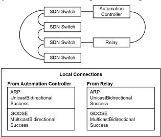
Fig. 4. SDN Logical Connections
