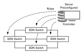
Fig. 3. Central Controller in an SDN Environment
