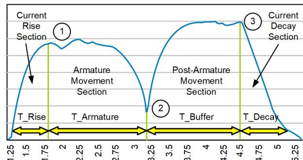
Fig. 4. Typical Trip Coil Current During an Operation
