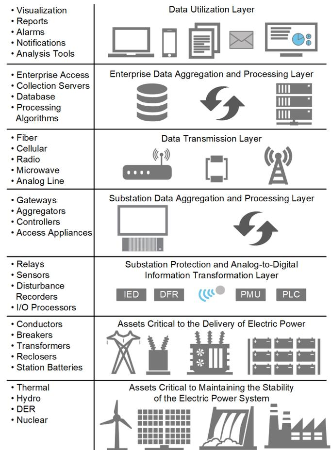
Fig. 1. Required Equipment, Functions, and Services
