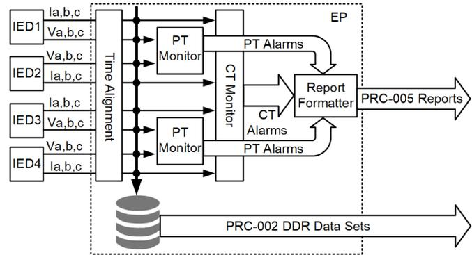
Fig. 3. Example PT/CT Monitoring System
