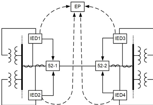
Fig. 2. Redundant PT/CT Topology
