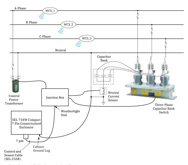
Figure C.4 Compact 7-Pin Connectorized Enclosure
