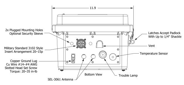
Figure 2.4 Bottom View of Connectorized Enclosure
