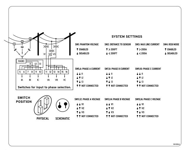
Figure 5.2 SEL-734W Control (DIP) Switch Settings
