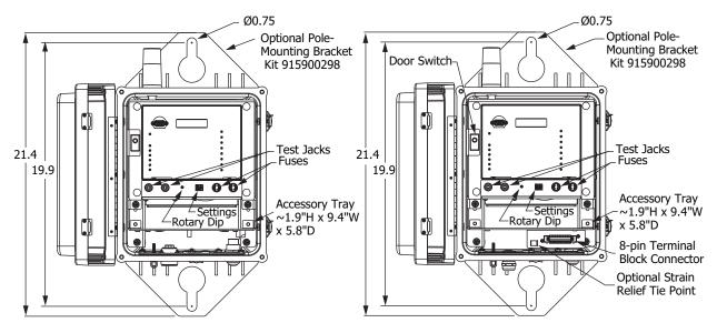
Figure 3.3 Compact 7-Pin Enclosure Mounting Dimensions
