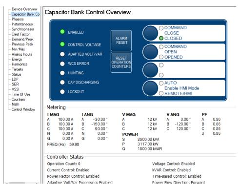
Figure 2.6 QuickSet HMI Capacitor Bank Control Overview
