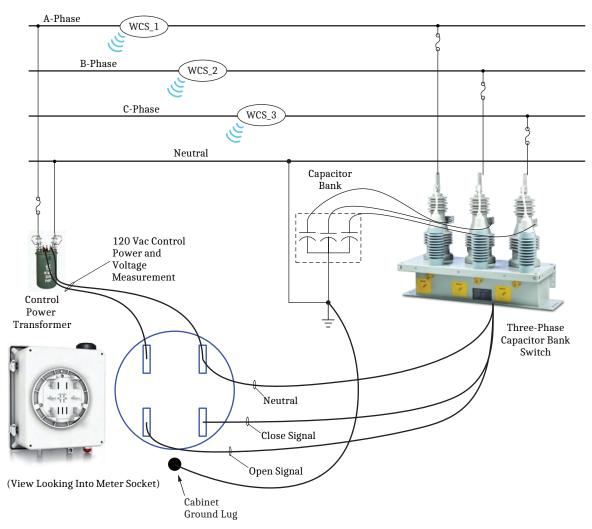
Figure C.5 Compact 4-Jaw Socket-Based Enclosure Connection Diagram
