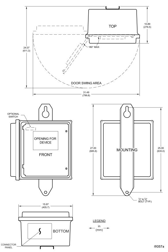
Figure 3.2 Full-Size Enclosure Mounting Dimensions
