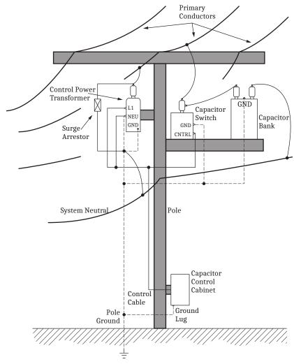
Figure 3.1 SEL-734W Required System Grounding
