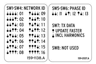
Figure 6.1 Control (DIP) Switch Configurations
