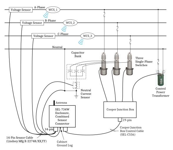
The Full-Size SEL-734W is not wired to use control power voltage for voltage measurement. If you would like to measure Phase A voltage from a CPT, you can make that connection in your junction box as seen in *Figure C.3*.
