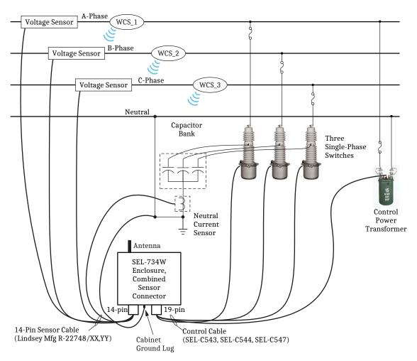
Figure 4.3 Three-Phase Measurements and Single-Pole Switching Application
