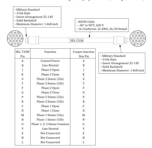
The SEL-C559 cable connects to a junction box as per Figure C.3 for end-user wiring.
