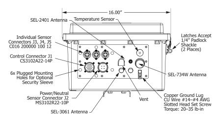
Figure 2.2 Bottom View of Enclosure With Individual Sensor Connectors
