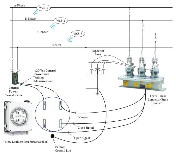
Figure C.8 Compact 4-Jaw Socket-Based Enclosure Connection Diagram
