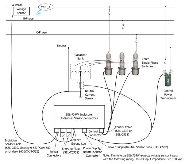
Figure C.6 Full-Size Enclosure With Individual Sensor Connectors (Installed With a Single Voltage Sensor and Generic Neutral Current Sensor)
