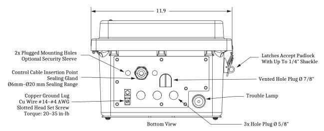
Figure 2.5 Bottom View of Terminal Block Enclosure
