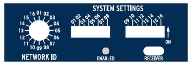
Figure 5.3 SEL-734W Wireless Receiver Panel
