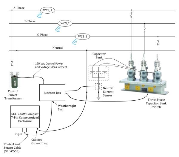
Figure C.7 Compact 7-Pin Connectorized Enclosure
