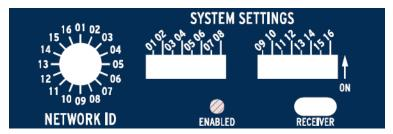
Figure 5.3 SEL-734W Wireless Receiver Panel
