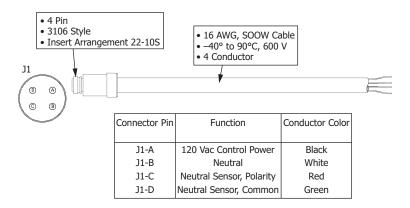
Cable SEL-C539 connects to one Lindsey Manufacturing neutral sensor and the control power transformer (4-pin male connector).
