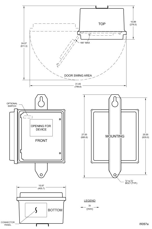
Figure 3.2 Full-Size Enclosure Mounting Dimensions
