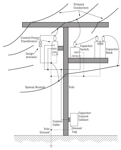
Figure 3.1 SEL-734W Required System Grounding
