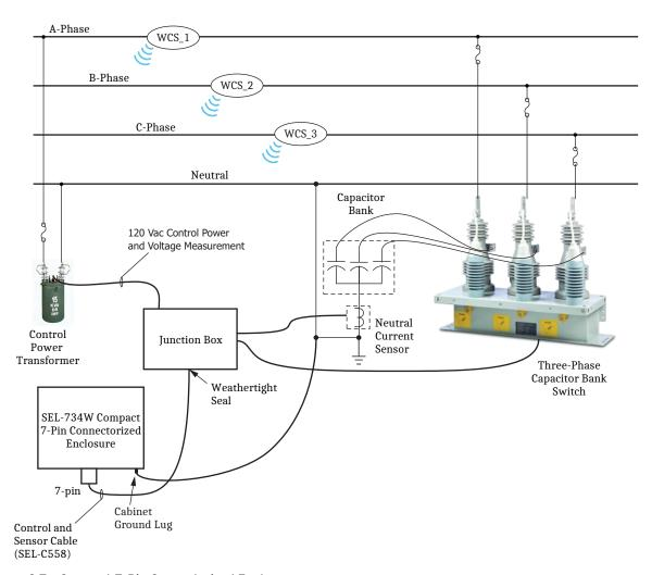
Figure C.7 Compact 7-Pin Connectorized Enclosure
