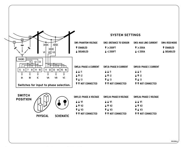
Figure 5.2 SEL-734W Control (DIP) Switch Settings
