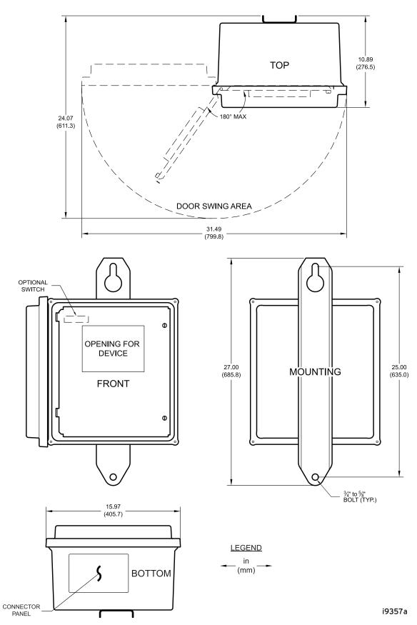
Figure 3.2 Full-Size Enclosure Mounting Dimensions
