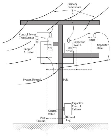
Figure 3.1 SEL-734W Required System Grounding
