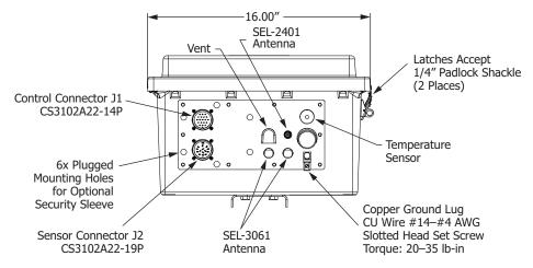
Figure 2.1 Bottom View of Enclosure With Combined Sensor Connector
