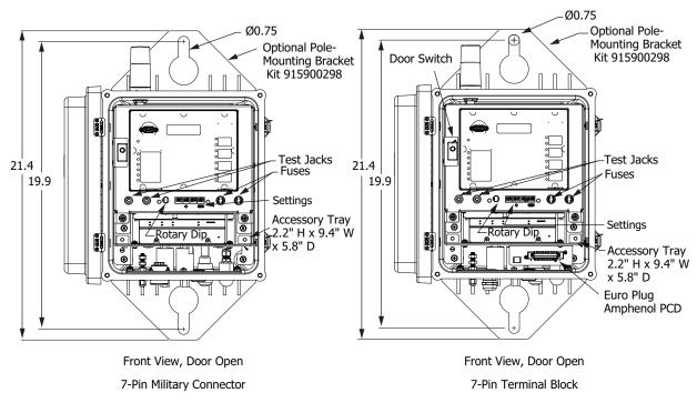
Figure 3.3 Compact 7-Pin Enclosure Mounting Dimensions
