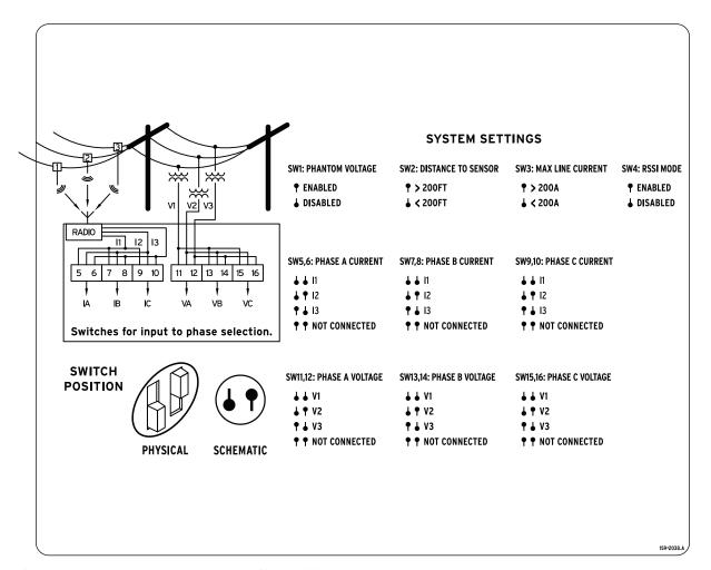
Figure 5.2 SEL-734W Control (DIP) Switch Settings
