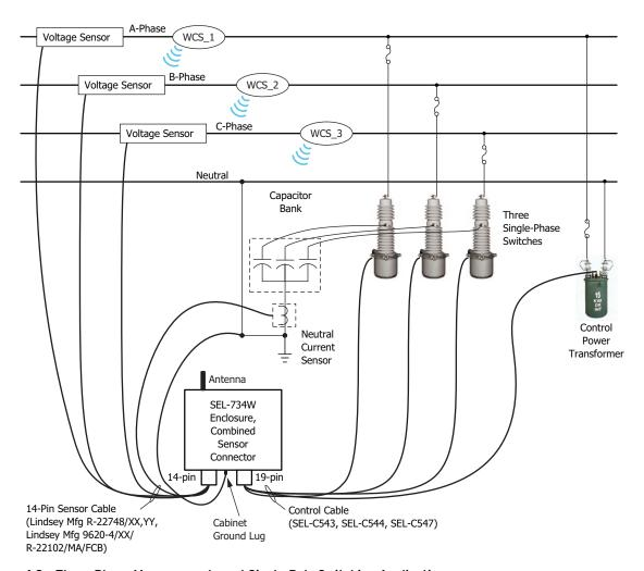
Figure 4.3 Three-Phase Measurements and Single-Pole Switching Application
