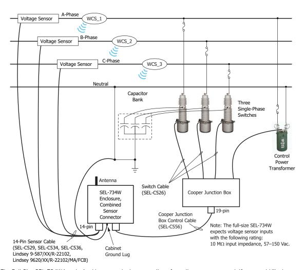
The Full-Size SEL-734W is not wired to use control power voltage for voltage measurement. If you would like to measure Phase A voltage from a CPT, you can make that connection in your junction box, as seen in *Figure C.3*.
