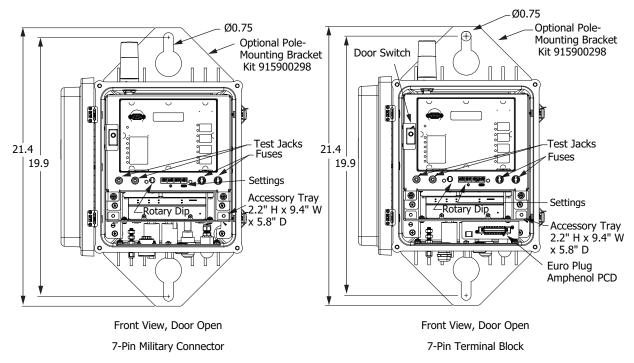
Figure 3.3 Compact 7-Pin Enclosure Mounting Dimensions
