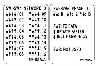
Figure 6.1 Control (DIP) Switch Configurations
