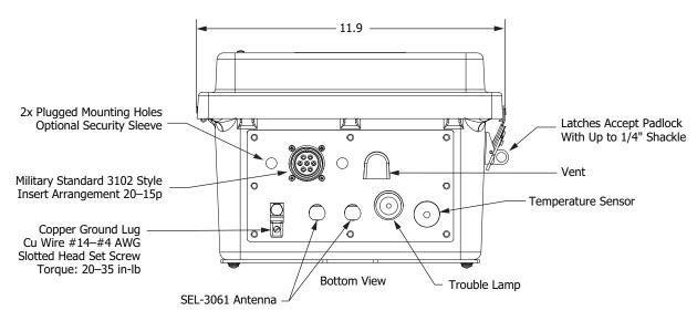
Figure 2.4 Bottom View of Connectorized Enclosure
