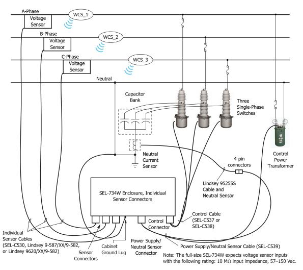
Figure C.5 Full-Size Enclosure With Individual Sensor Connectors (Installed With a Lindsey Neutral Current Sensor)
