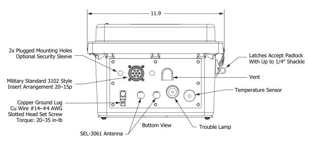
Figure 2.4 Bottom View of Connectorized Enclosure
