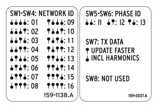
Figure 6.1 Control (DIP) Switch Configurations
