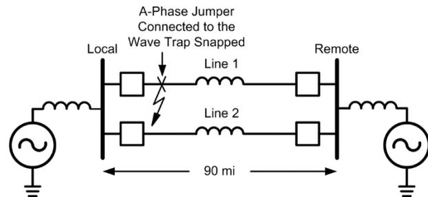
Fig. 25. Broken-conductor field event in a parallel-transmission-line system.
