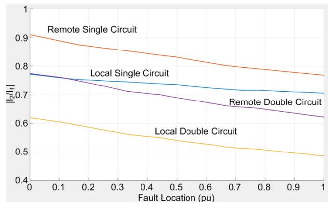
Fig. 16.  $|I_2/I_1|$  for broken-conductor faults over the length of the line for single-circuit and double-circuit models.
