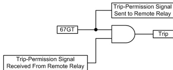
Fig. 18. POTT scheme used for line protection.
