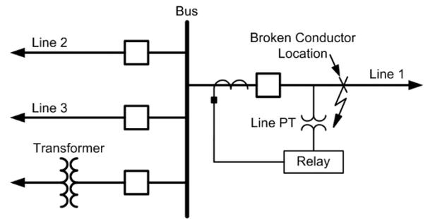
Fig. 8. One-line diagram of a typical transmission substation with a close-in broken-conductor fault on Line 1.
