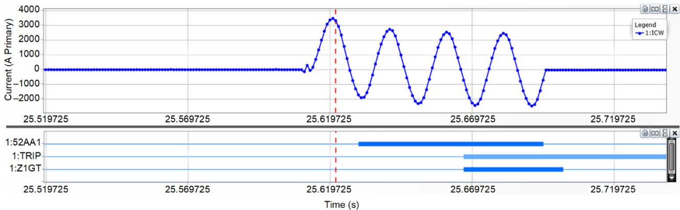
Fig. 21. Fault-current waveform when the breakers were closed on the fault from the remote end.
