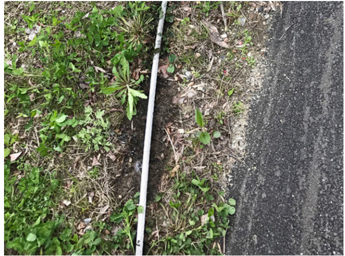
Fig. 15. Staged HIF Test 1 showed arcing on the grass following the test.
