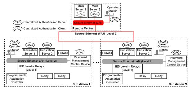
Fig. 1. Typical power network architecture with sample APM system.
