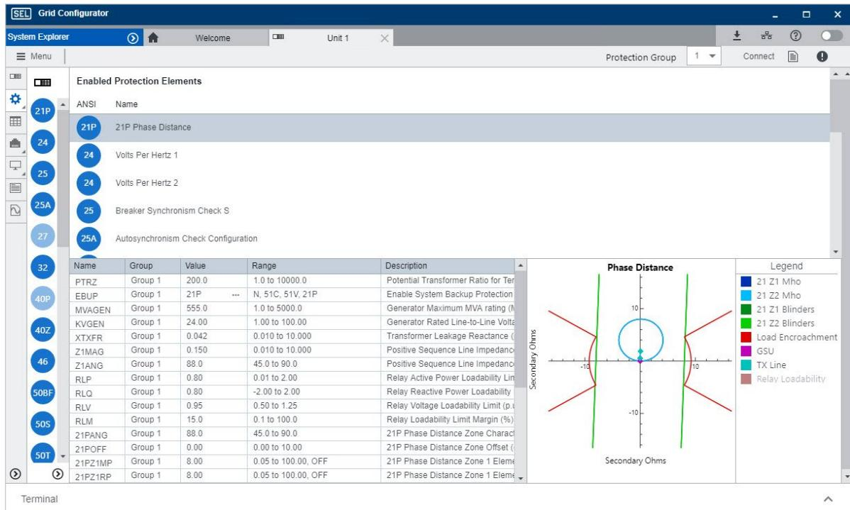
The SEL Grid Configurator visualization tools help you easily adjust device protection elements.
