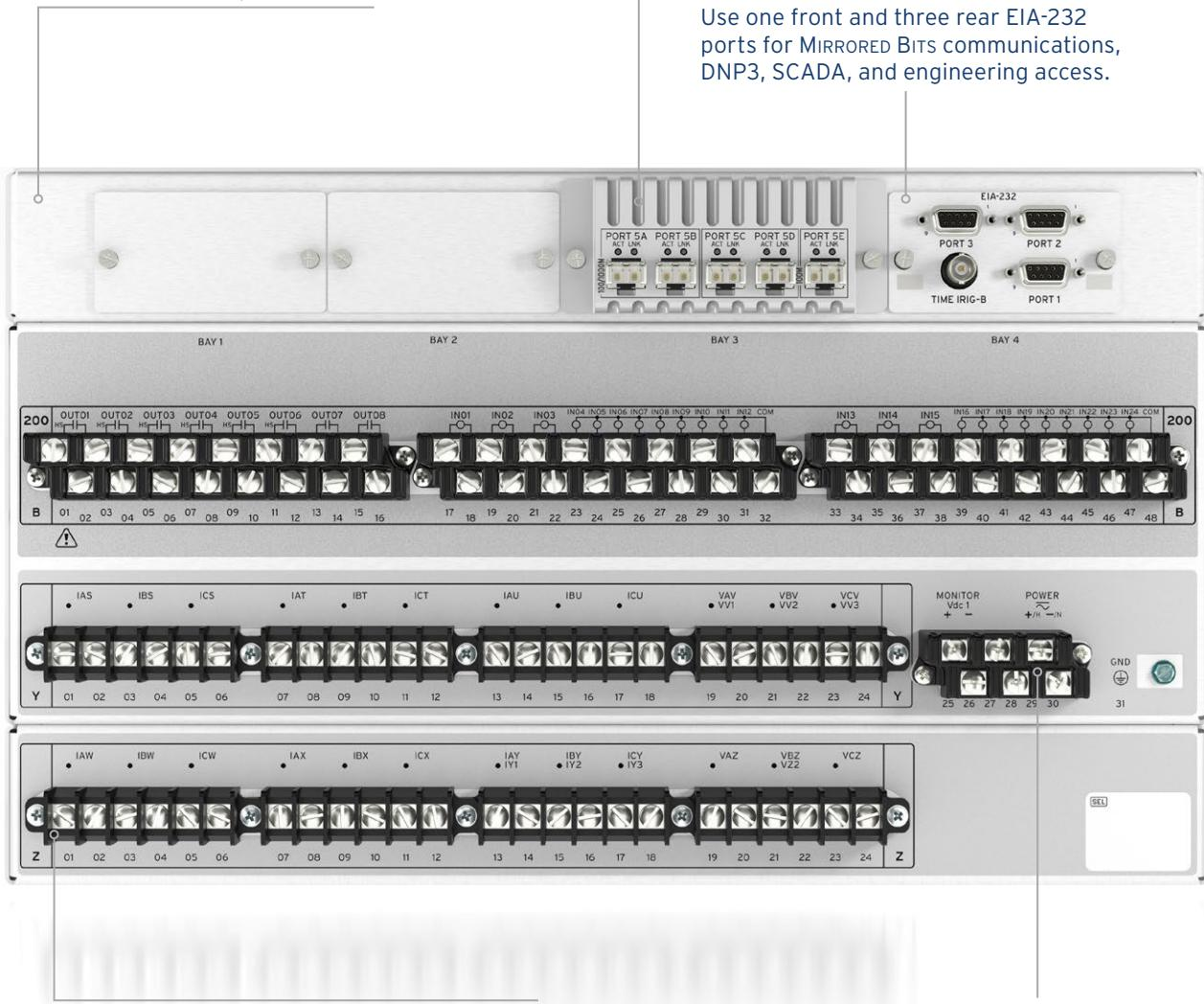
The 18 current and 6 voltage channels support differential protection for up to 6 three-phase terminals, 3 independent REF elements, and voltage elements.
