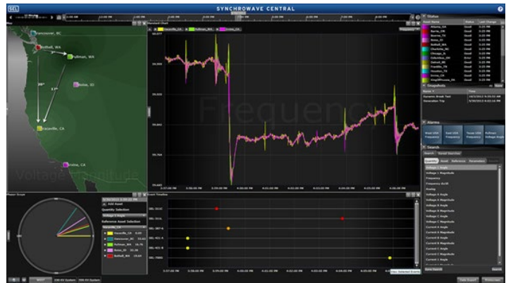
Monitor grid conditions with time-aligned synchrophasor messages.
