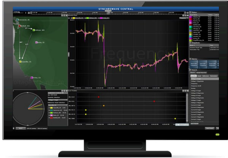
Monitor grid conditions with time-aligned synchrophasor messages.
