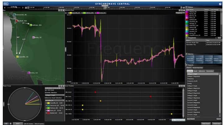
Monitor grid conditions with time-aligned synchrophasor messages.
