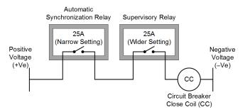
Fig. 4 Two Sync-Check Relays in Series
