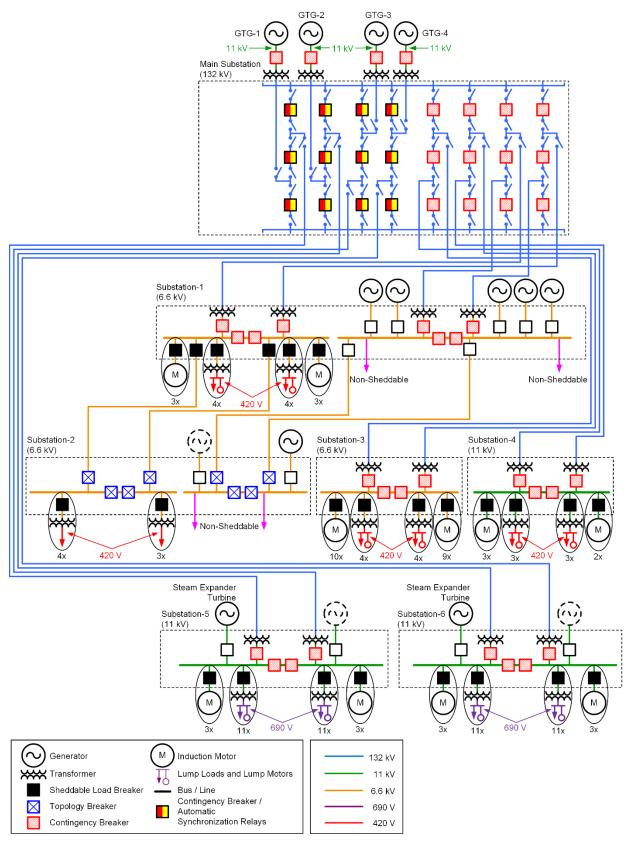
Fig. 1 Simplified One-Line Diagram
