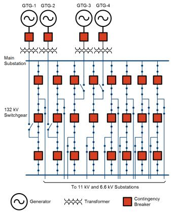
Fig. 2 GCS Simplified One-Line Diagram
