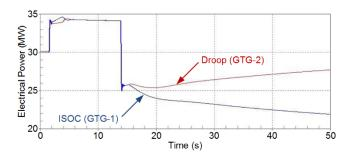
Fig. 8 Electrical Power Comparison of GTG-1 Unit Versus GTG-2 Unit for Loss of 9 MW Expander Generator and Level-1 Underfrequency
