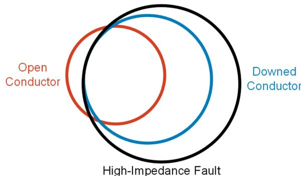
**Figure 4 HIFs vs. Downed Conductors**
