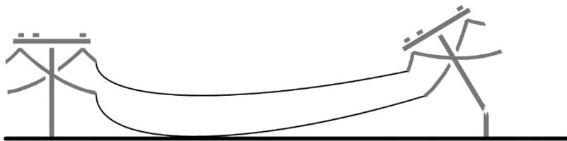
Figure 1 Downed Conductor
