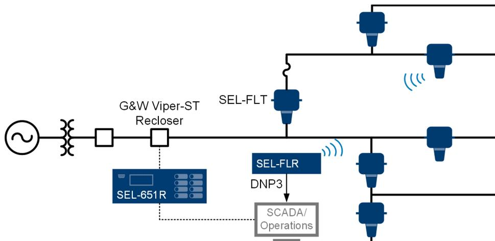
**Figure 5 Example SEL-FLT and SEL-FLR Application**
