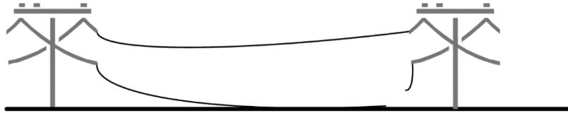
**Figure 2 Downed Broken Conductor**
