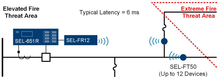
**Figure 7 Dynamic Reclosing Application Using the SEL-FT50 and SEL-FR12**
