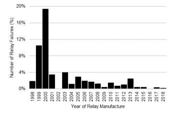
Fig. 3. The number of relay failures recorded by Utility A versus year of manufacture.
