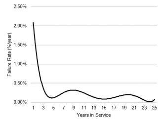
Fig. 1. Field-observed reliability life cycle of a 1992-vintage transmission relay manufactured between 1992 and 1999.
