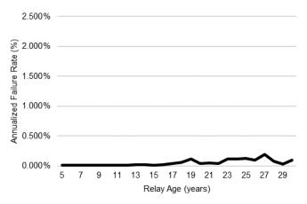
Fig. 2. Annualized failure rate by relay age for relays returned to the manufacturer in 2018.
