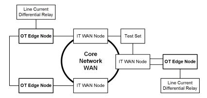
Figure 3 Performance Test Network Topology
