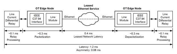
Figure 5 Live Line Current Differential Circuit Substation Results
