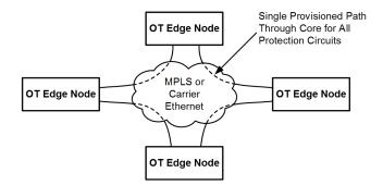
Figure 2 VSN Ring Topology Supported by Static Paths Through Core
