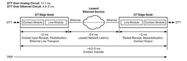
Figure 4 Live DTT Circuit Substation Results
