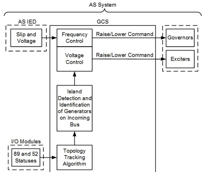
Fig. 6. Autosynchronization Control System
