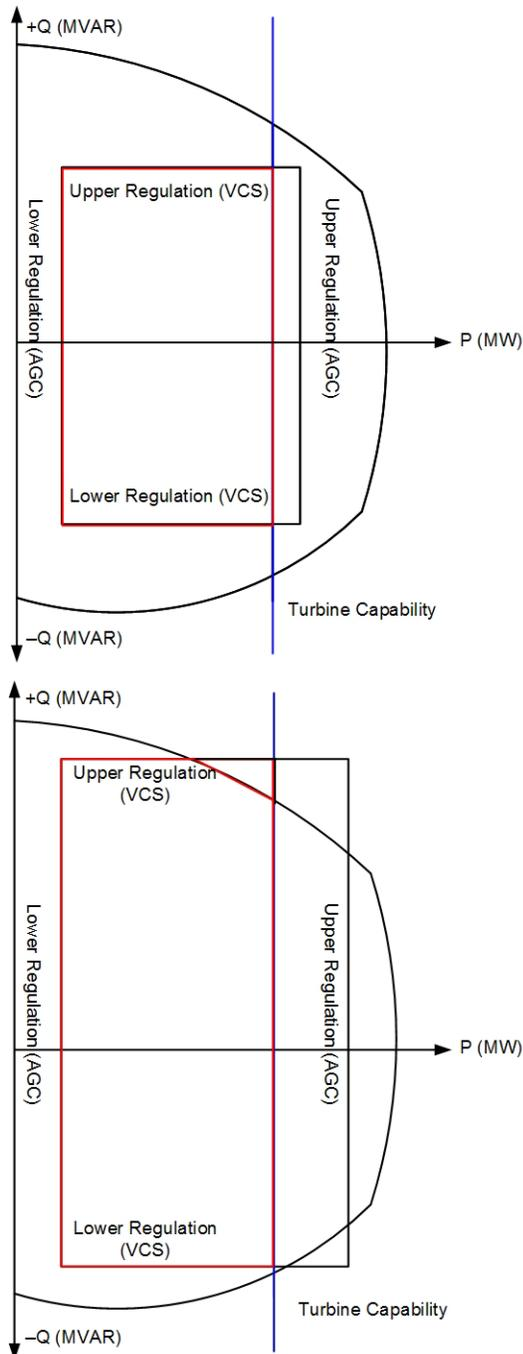
Fig. 5. Generator Capability – Regulation Limits With Generator Boundary
