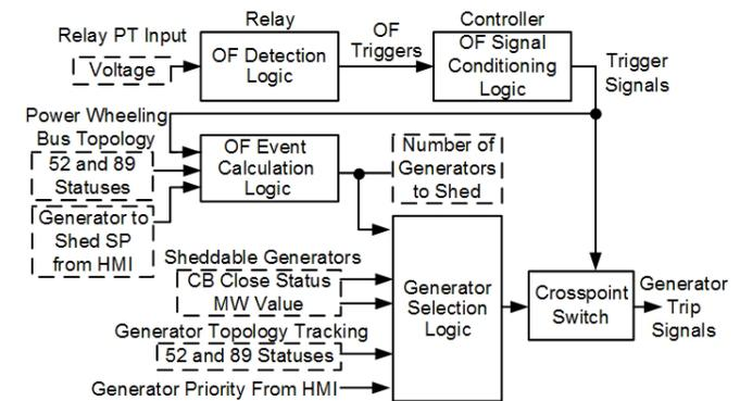
Fig. 9. OFGS System Algorithm
