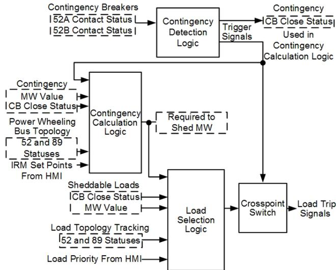
Fig. 7. CLS System Algorithm
