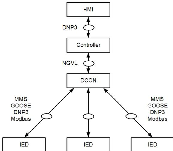
Fig. 2. PMCS System Architecture with Data Flow Paths
