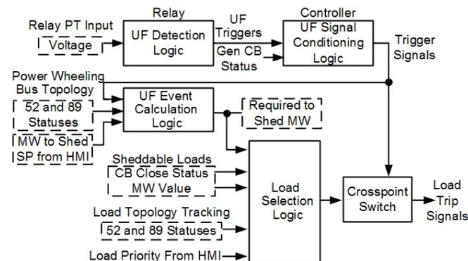
Fig. 8. UFLS System Algorithm
