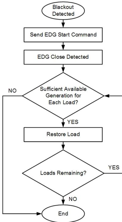
Fig. 10. EBS System Logic Flow
