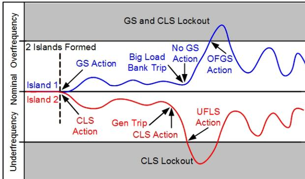
Fig. 11 Example Simulation Result
