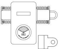
Ensure that the conductor is energized and the minimum load current has been present for at least three minutes. Hold the CRSRTT tool against the bottom right side of the housing for at least 15 seconds. Remove the tool to complete the trip or reset process.
