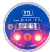
Permanent fault indication.
