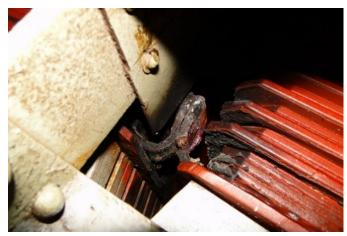
Fig. 26. LOF condition resulting from open-circuited field winding.
