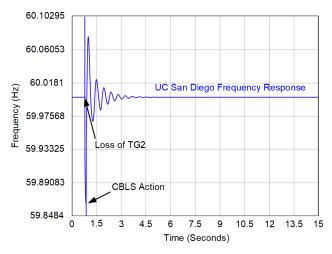
Fig. 14. Case B: Loss of Generation at Station B
