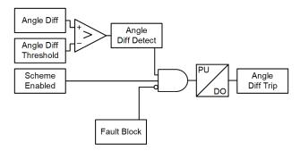
Fig. 8. Wide-Area Angle-Based Detection
