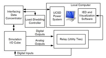
Fig. 11. RTDS Closed-Loop Interface
