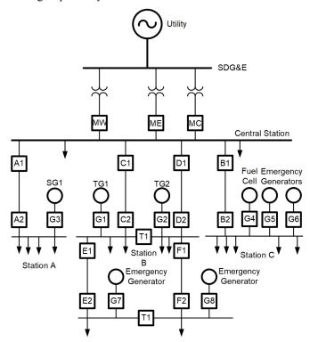
Fig. 1. UC San Diego Simplified One-Line Diagram
