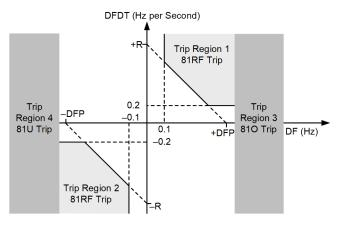
Fig. 7. Decoupling Scheme Characteristics
