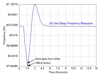
Fig. 12. Case A: Islanding for Grid Disturbance
