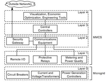
Fig. 2. High-Level Microgrid Architecture
