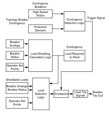
Fig. 4. Contingency-Based Load-Shedding Algorithm
