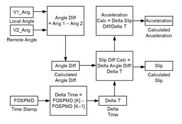
Fig. 9. Wide-Area Parameter Calculation
