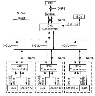
Fig. 3. Microgrid Communications Network
