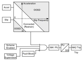
Fig. 10. Slip- and Acceleration-Based Wide-Area Scheme
