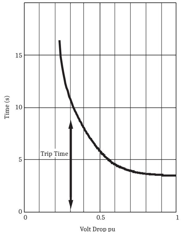
**Figure 5** VAR-Flow Controlled Time Undervoltage Load Shedding
