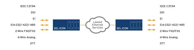
You can combine ICON deterministic transport with dedicated analog drop interfaces, including 2-wire FXO/FXS, 4-wire analog voice frequency, and DTT. These interfaces allow you to preserve existing analog end equipment and create a low-latency circuit through your digital leased line to maintain end-to-end communications channel performance for critical applications. With the ICON, you can achieve end-to-end latency of less than 5 ms for a contact transfer across leased Ethernet service.
