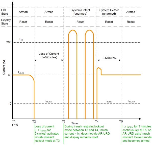
Figure 2 Response of AR-URD to Inrush Currents Falsely Appearing as Fault Currents
