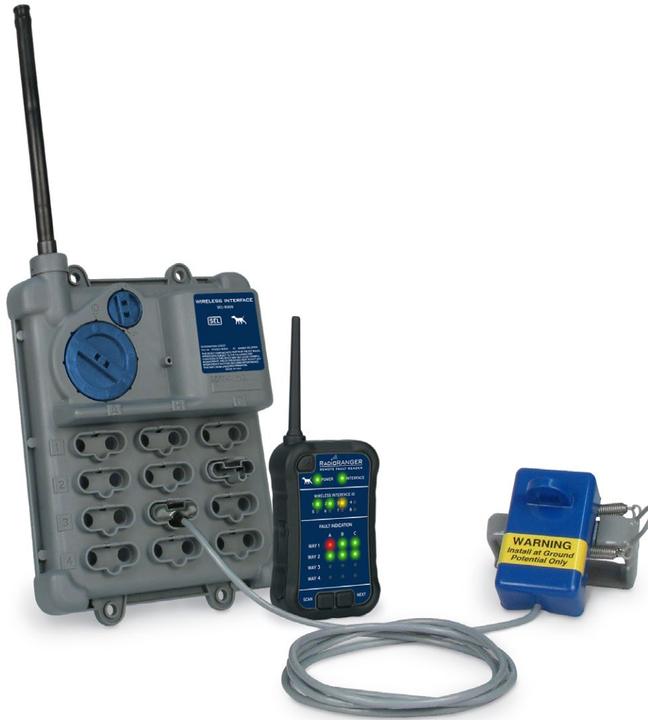
Figure 5: RadioRANGER Wireless Fault Indication System Option (SEL-8300 Wireless Interface, SEL-8310 Remote Fault Reader, and SEL AR-URD Fault Indicator connected by magnetic interface probe).
