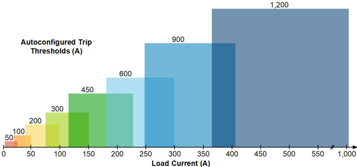
Figure 1 Autoranging Graph Used by AR-URD to Configure Trip Threshold
