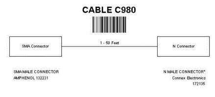
CABLE: RG-8X Coaxial cable with braided shield and PVC jacket
