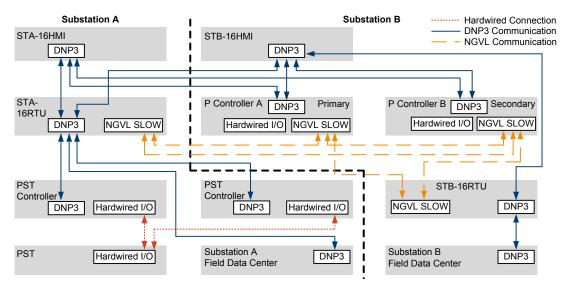
Figure 1. Data Flow Diagram (DFD) of P Control System
