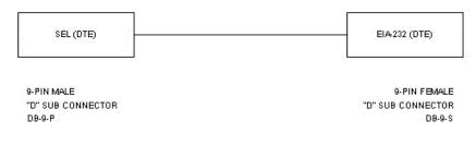
CABLE: 8 Conductor 22 AVVG 7/30 Tinned Copper with PVC Jacket (Shielded: Alpha 1298C or equal)
